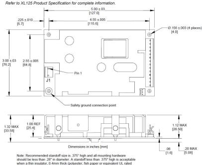
94V-2 minimum) is placed between the XL125 and the mounting chassis (refer to applicable UL standard for clearance requirements)
