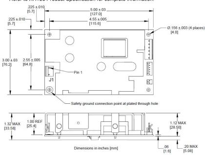
Note: Recommended standoff size is .375" high and all mounting hardware should be less than .28" in diameter. A standoff less than .375" high is acceptable thin insulator, 0.4mm thick (polyester, fish paper or equivalent UL rated 94V-2 minimum) is placed between the XR125 and the mounting chassis (refer to applicable UL standard for clearance requirements).
